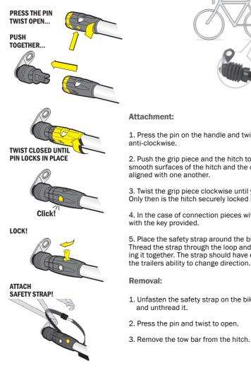
1. Press the pin on the handle and twist the grip piece
